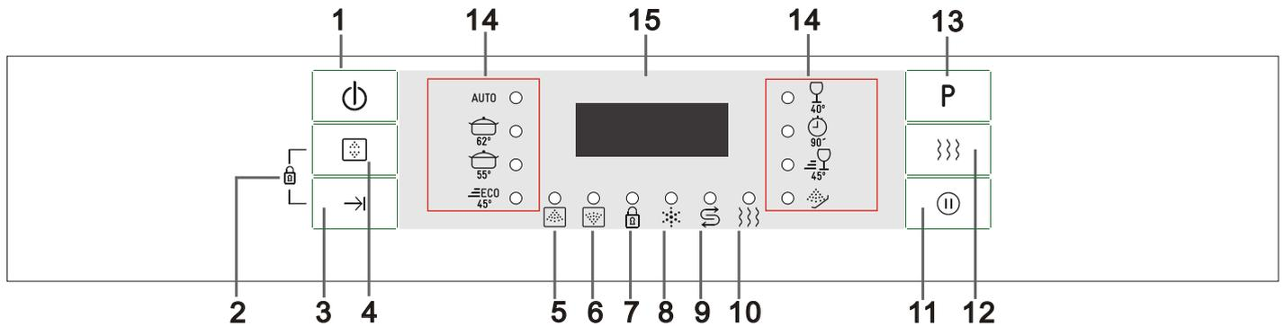
1. On/Off Button: to switch On/Off the appliance;
