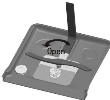
Step 1: Turn the filter in anti-clockwise direction,
