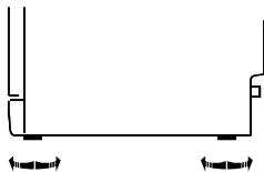
Once the appliance is positioned for levelling, the height of the dishwasher may be altered via adjustment of the screwing level of the feet.
